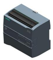
SIMATIC S7-1200, CPU 1214C, compact CPU, DC/DC/DC, onboard I/O: 14 DI 24 V DC; 10 DO 24 V DC; 2 AI 0-10 V DC, Power supply: DC 20.4-28.8V DC, Program/data memory 100 KB
