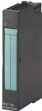
SIMATIC DP, Electronics module f. ET200S, 2AI Standard I-4DMU 15 mm width, +/-20mA; 13 bit+sign 4.. 20mA; 12-bit for 4-wire transmitter Cycle time 65 ms/channel with SF LED (group fault)
