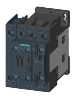
4NO CONTACTOR, AC1: 40A AC 230V 50HZ 4-POLE, 4NO, SZ: S0, SCREW TERMINAL 1NO+1NC INTEGR.
